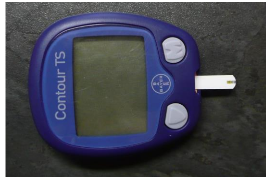
The glucometer strip is in the meter but not pushed in fully (you know this because the display is off)
